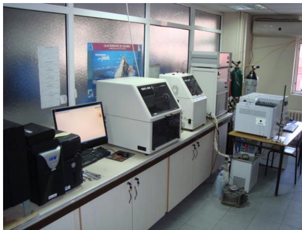
Fig 1. In the Lab - Integrated Microreactor-MS, with CATLAB-PCS Module & QIC-20 MS Module
