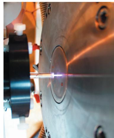
Fig 1. Atmospheric plasma produced between the RF electrode, or needle, and the sampling orifice of the Hidden Molecular Beam Mass Spectrometer.
