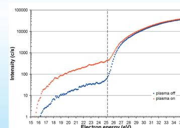
Fig 8. Appearance potential scans for N with the plasma on and off. The threshold for the dissociative ionisation from N<sub>2</sub> is 25.2eV.
