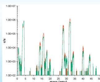
Fig 6. Neutral mass spectra for plasma on (red trace) and plasma off or background (green trace).
