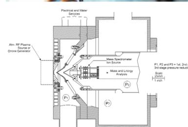
Fig 2. Schematic of the Hidden Modulated Beam Mass Spectrometer System. The three cones are fitted with apertures of 0.2mm at the first stage, 0.3mm at the second stage and 1.0mm at the entrance of the EQP mass/energy analyser.
