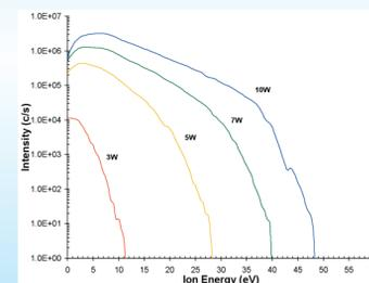
Fig 5. Ion energy distributions for O<sup>+</sup> from the He/O<sub>2</sub> plasma as a function of discharge power.
