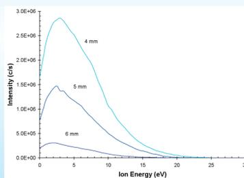
Fig 4. Ion energy distributions for N<sup>+</sup> from the He/N<sub>2</sub> plasma as a function of distance from the sampling orifice.
