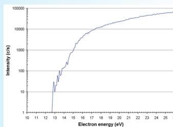
Fig 9. Appearance potential of O<sub>3</sub><sup>+</sup> produced in a commercial ozone generator.
