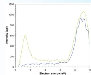
Fig 10. O<sub>2</sub><sup>-</sup> produced by electron attachment in the EQP ion source when the ozone generator is on (green line) and when it is off (blue line).
