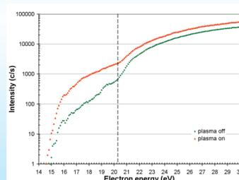
Fig 7. Appearance potential scans for O with the plasma on and off. The threshold for the dissociative ionisation of O<sub>2</sub> is 20.3eV.
